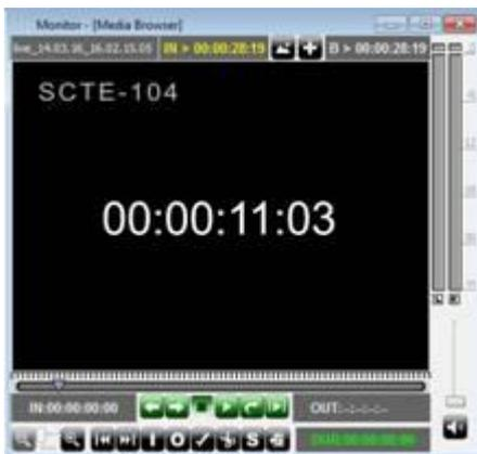
The window File Monitor of the application Air Manager allows viewing the record frame-by-frame, define the presence of VANC-batches, check the presence and the positions of messages in the recorded signal. Activation of the mode for displaying the VANC-batches is implemented in the menu for configuring Air Manager: **File-> Configure-> Preview-> item Show ANC.**
